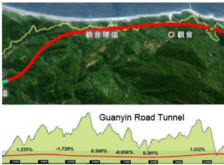
Fig.1 The geographical location and elevation of the Guanyin Road Tunnel (觀音隧道) in the Taiwan No. 9 Su-Hua Highway.
